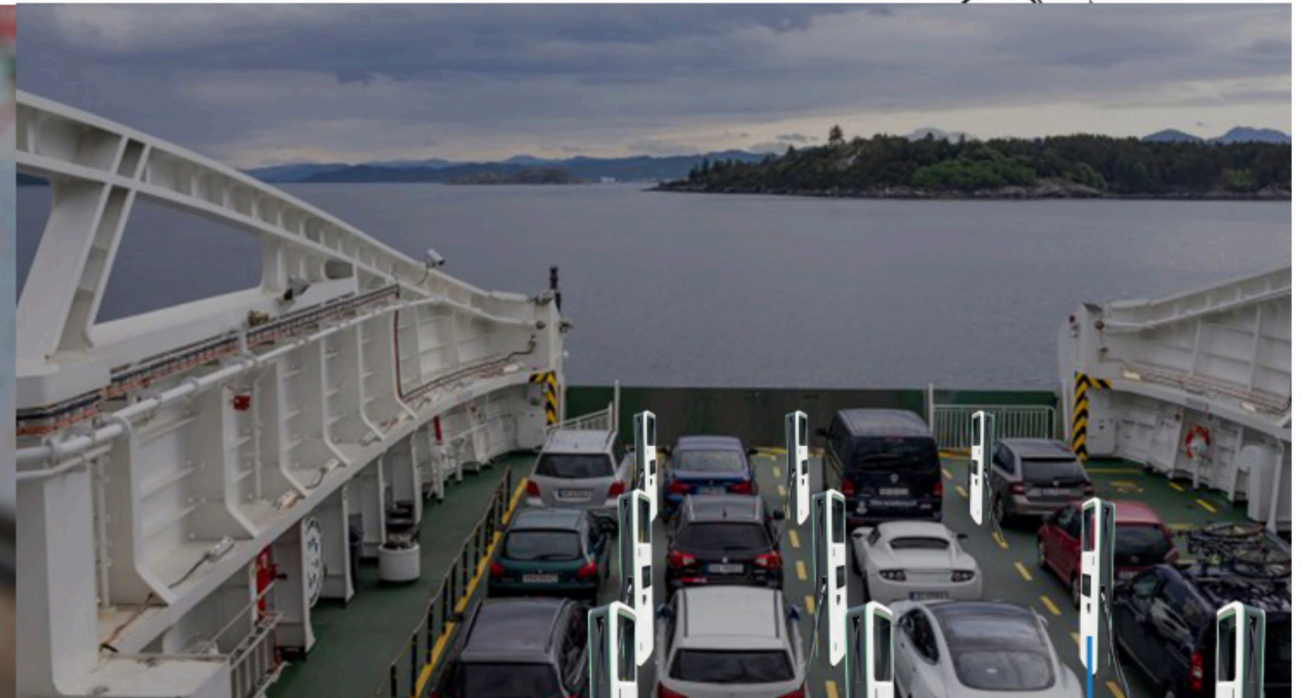
Each spot on the ferry is equipped with the potential to charge at a Level 2 (5kW), Level 3 (80kW) or Level 4 (120kW) capability. Prices vary by charging level and by charging time.
